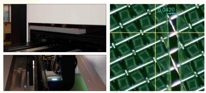
The high-definition DMD chip with 4° technology for perfect edge sharpness and long-lasting lasers exposes each pixel up to 800 times for even and optimal cross-linking of the emulsion.
